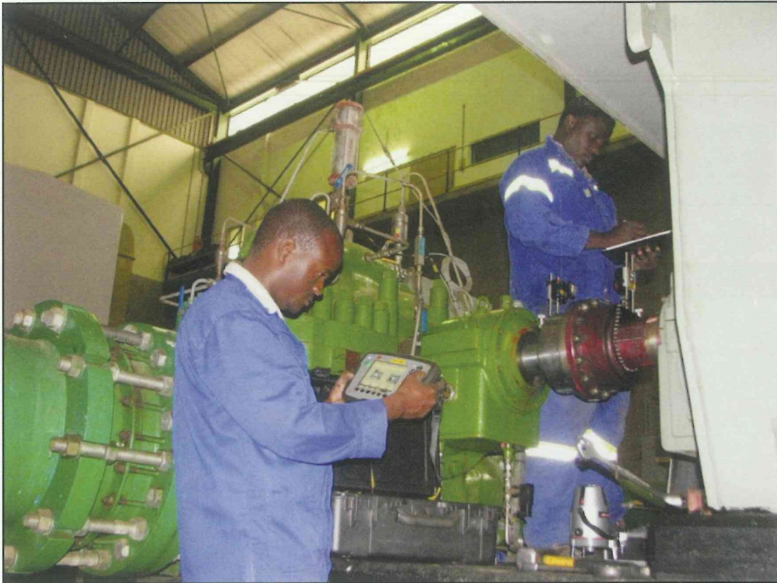
The artisan Mr Nelson Mokwala and his assistant Mr Kenneth Moloto doing laser alignment on pumps.
