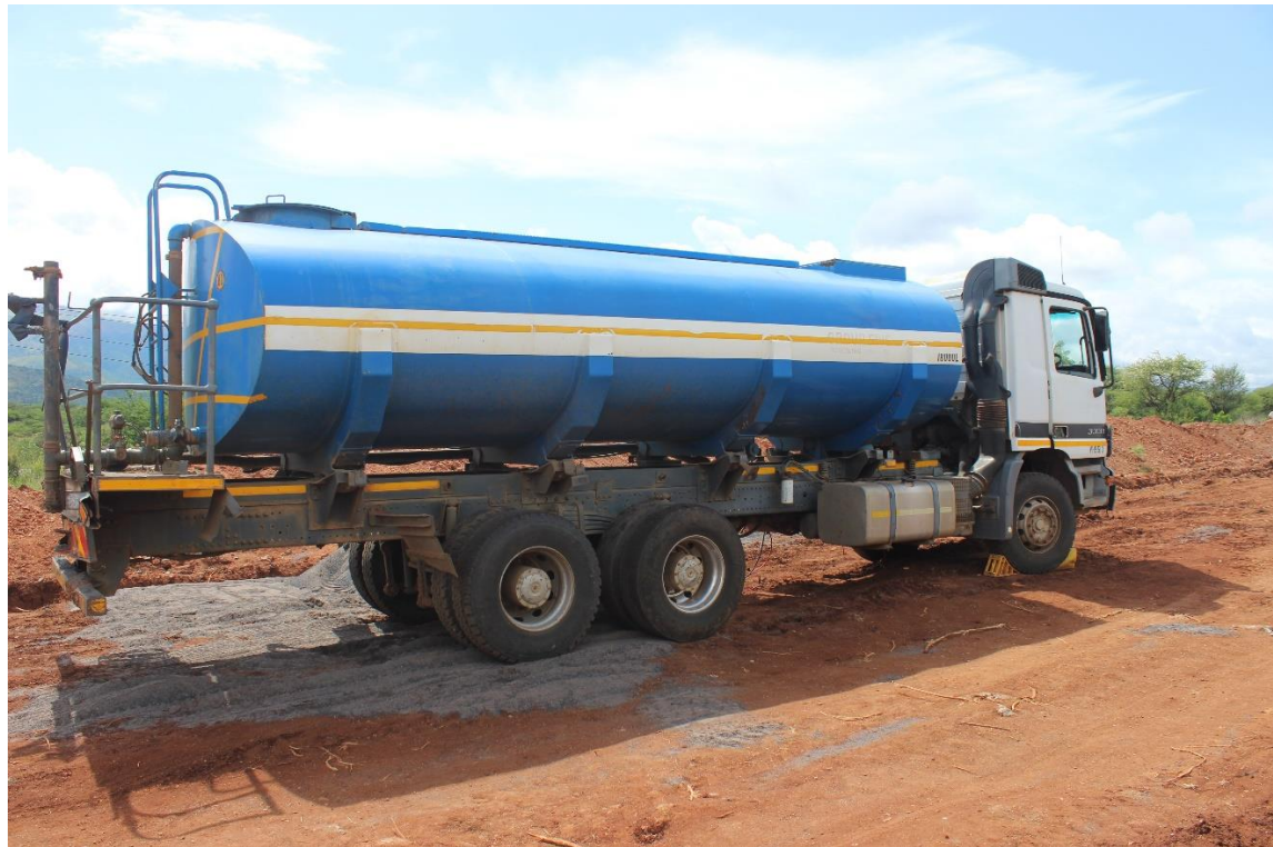
Photo 34: Water Bowser Tank at the pipeline
