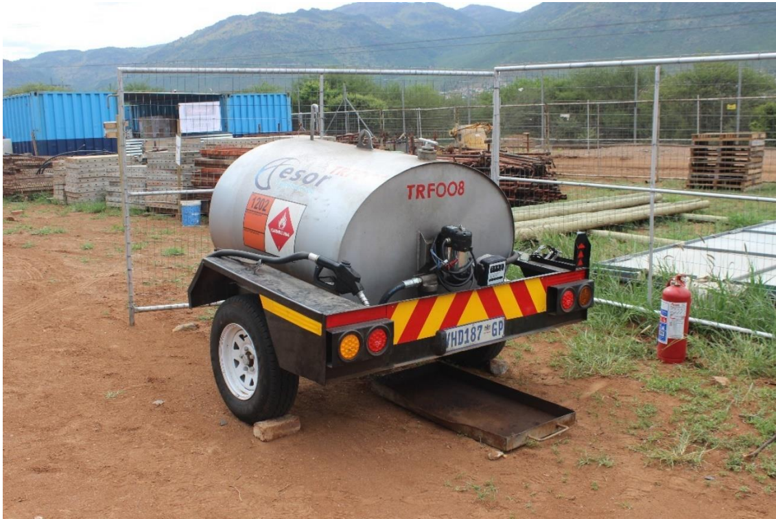
Photo 23: Drip trays under machinery not in use at the Spitskop Pump Station
