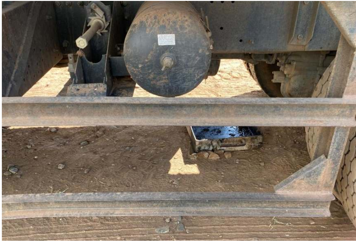
Photo 25: Drip trays under machinery not in use.
