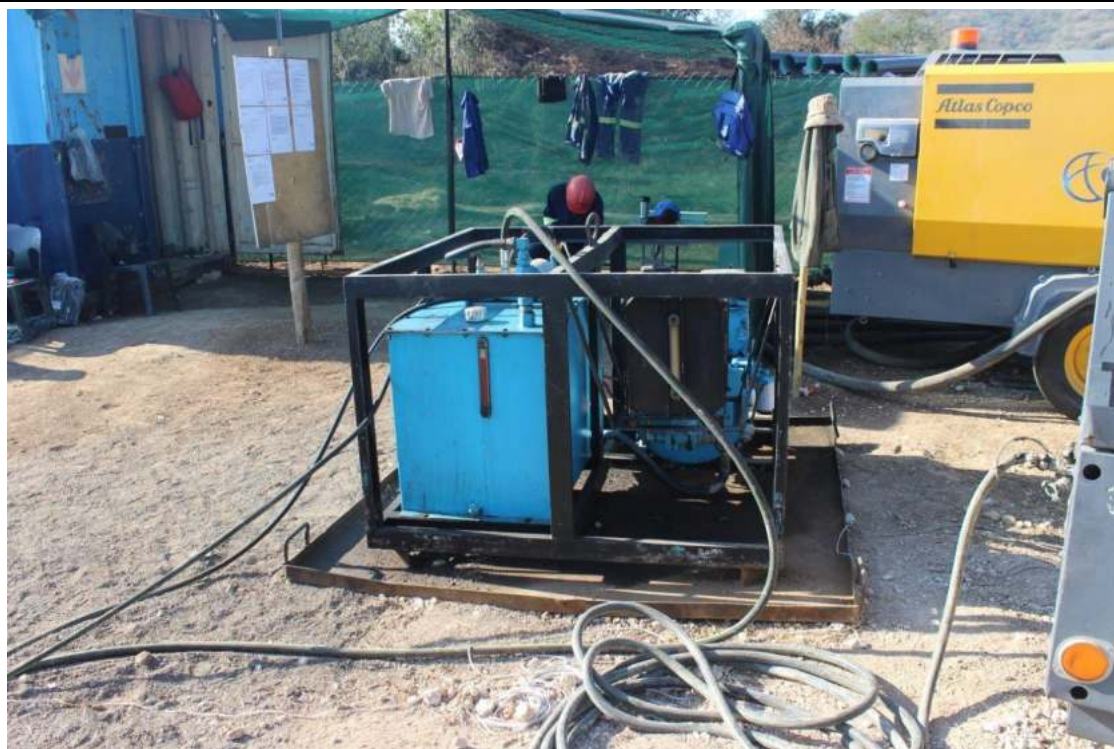
Photo 26: Drip trays under machinery not in use.
