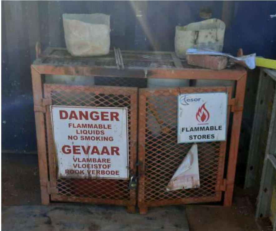
Photo 31: Chemical Storage Cage Locked
