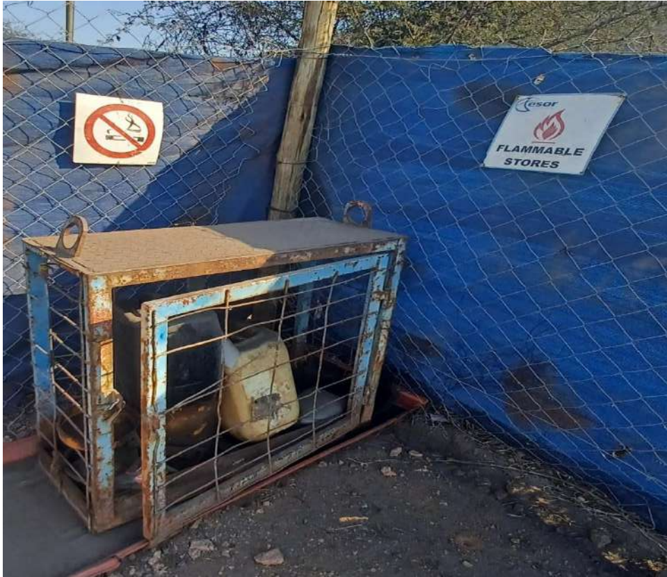
Photo 41: Chemical Storage Cage Unlocked and MSDS Sheet
