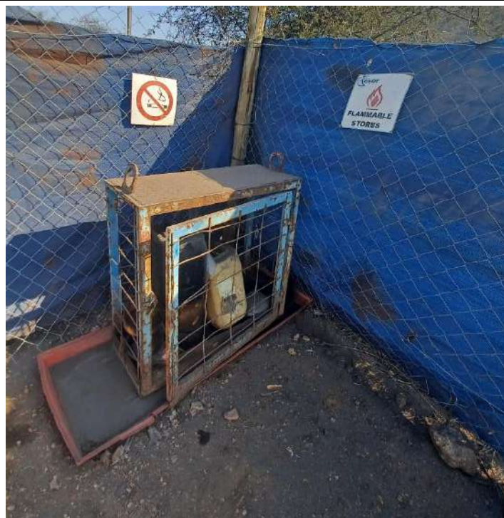
Photo 34: Drip trays used on site
