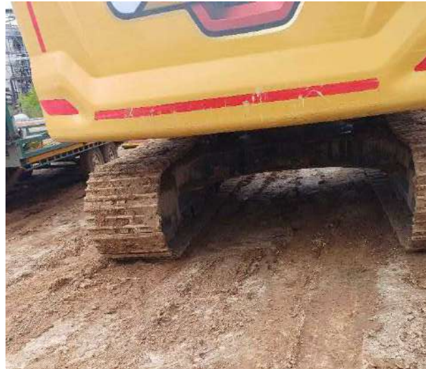
Photo 35: Drip trays not found under machinery on site
