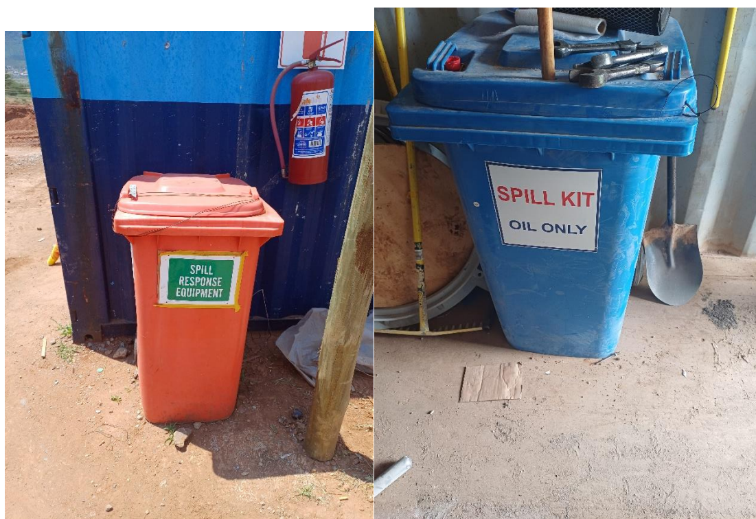
Photo 36: Hydrocarbon spill kits on site
