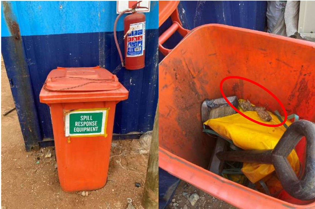
Spill kit being used as a waste bin
