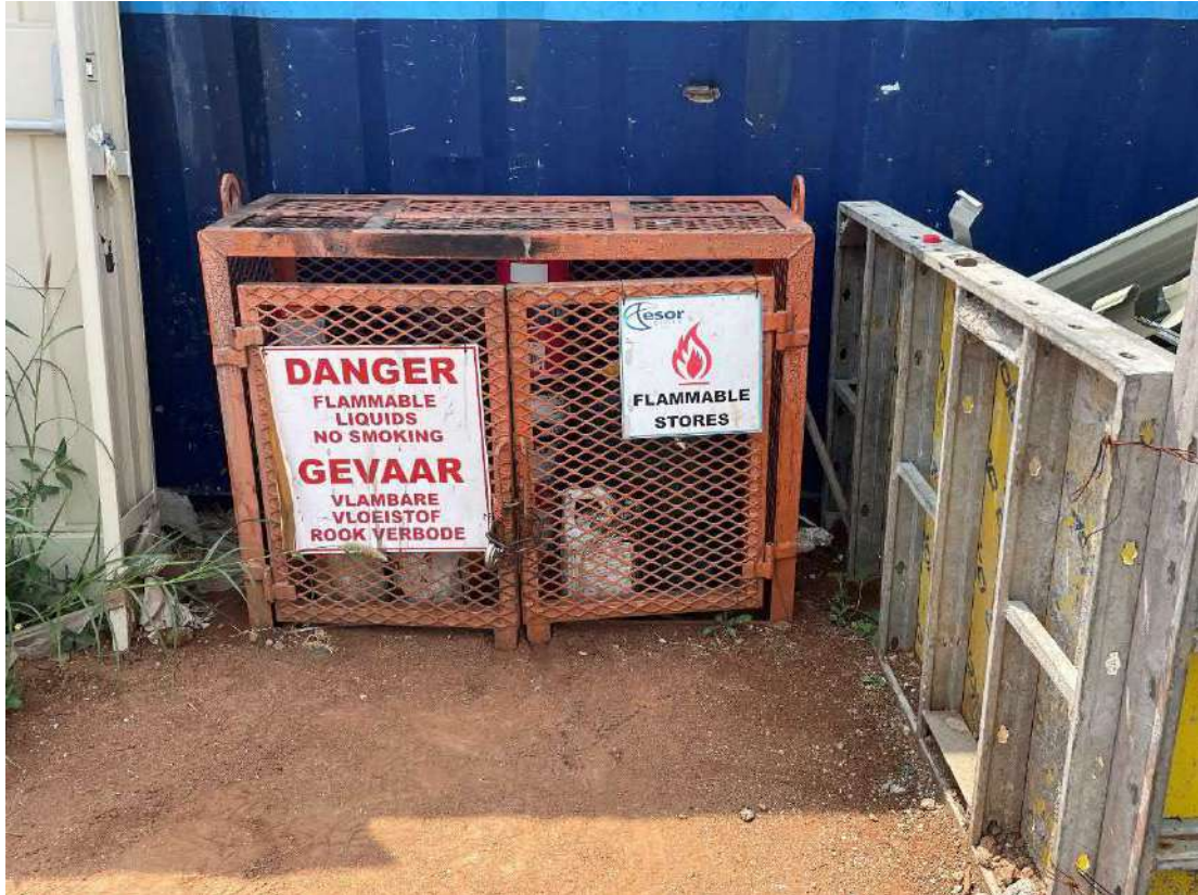
Photo 39: Chemical Storage Cage unlocked
